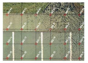
Points on a grid and intelligent SmartPick snaps provide a highly productive automated surveying tool used to create COGO points most typically used to generate a ground surface\TIN.
